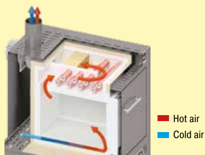
Schematic presentation of air circulation in ashing furnace L 24/11 BO
