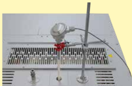
Thermocouple port in the ceiling with tripod
