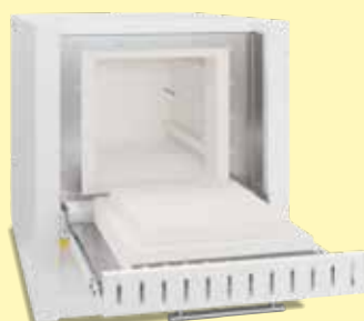
Muffle furnace LE 14/11
