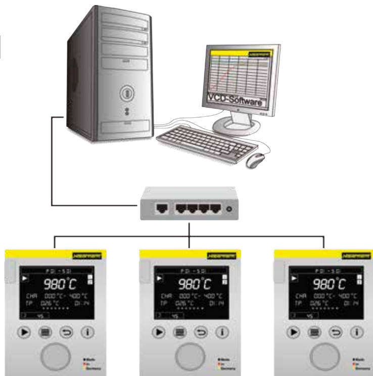
Example lay-out with 3 furnaces
