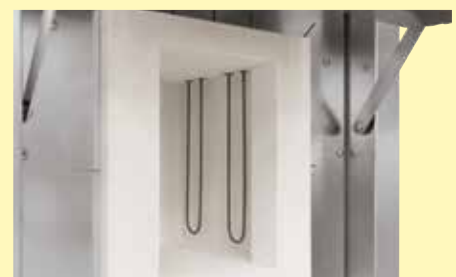
High-quality molybdenum disilicide heating elements
