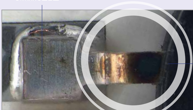
Soldered Led Pin - SZP-8 with iris diaphragm module and ST-156 stand.
