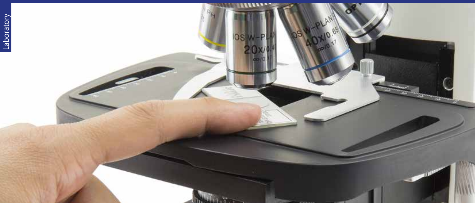
M-1140 Standard mechanical stage; 175x145mm for B-1000
