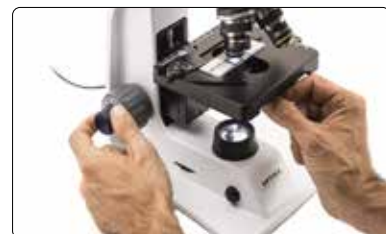
Regulation of diaphragm aperture
