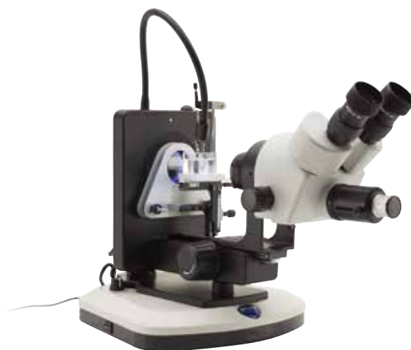
Horizontal position for immersion gem analysis
