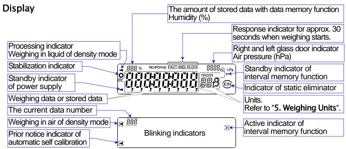
The interval memory function is used to store periodical weighing data. Refer to "12. Data Memory".
