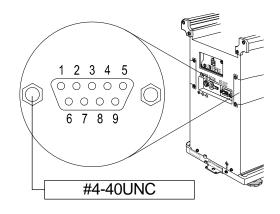
Signal names of the balance side are the same as the DTE side with TXD and RXD reversed.
