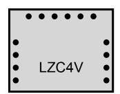
The LZC-4V photoreactor is equipped with 6 top lamps, and 8 side lamps.
